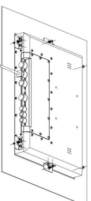
Step 3: Install the four remaining brackets. One on the left, one on the right, and two on top.
