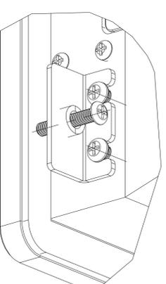
Step 4: Tighten the shorter M4x8mm screws to secure the bracket and tighten the longer M4x20mm screws to secure the monitor against the panel.
