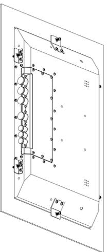
Step 3: Install the four remaining brackets. One on the left, one on the right, and two on top.
