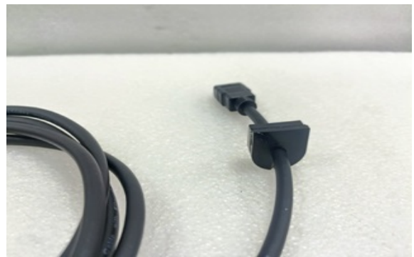
P4. Install Rubber Grommet onto HDMI cable.
