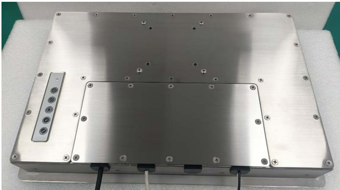
P6. Please ensure that the Rubber Grommets are pushed to the very bottom in order to guarantee the best water protection.
