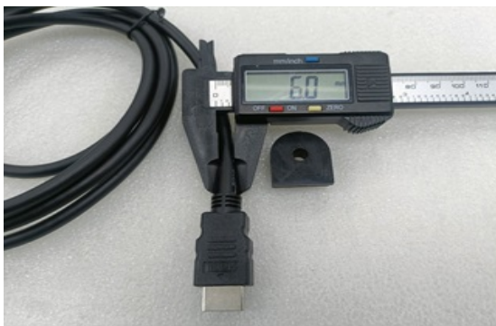
P3. Diameter of HDMI cable: 6mm.
