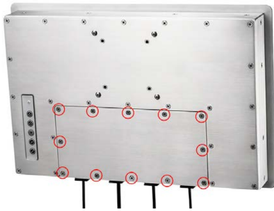
P1. Remove 12 Screws holding the cover
